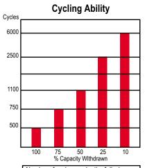
Number of cycles vs. depth of discharge at +20°C discharge with 20 hour rate
