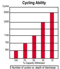
at +20°C discharge with 20 hour rate
